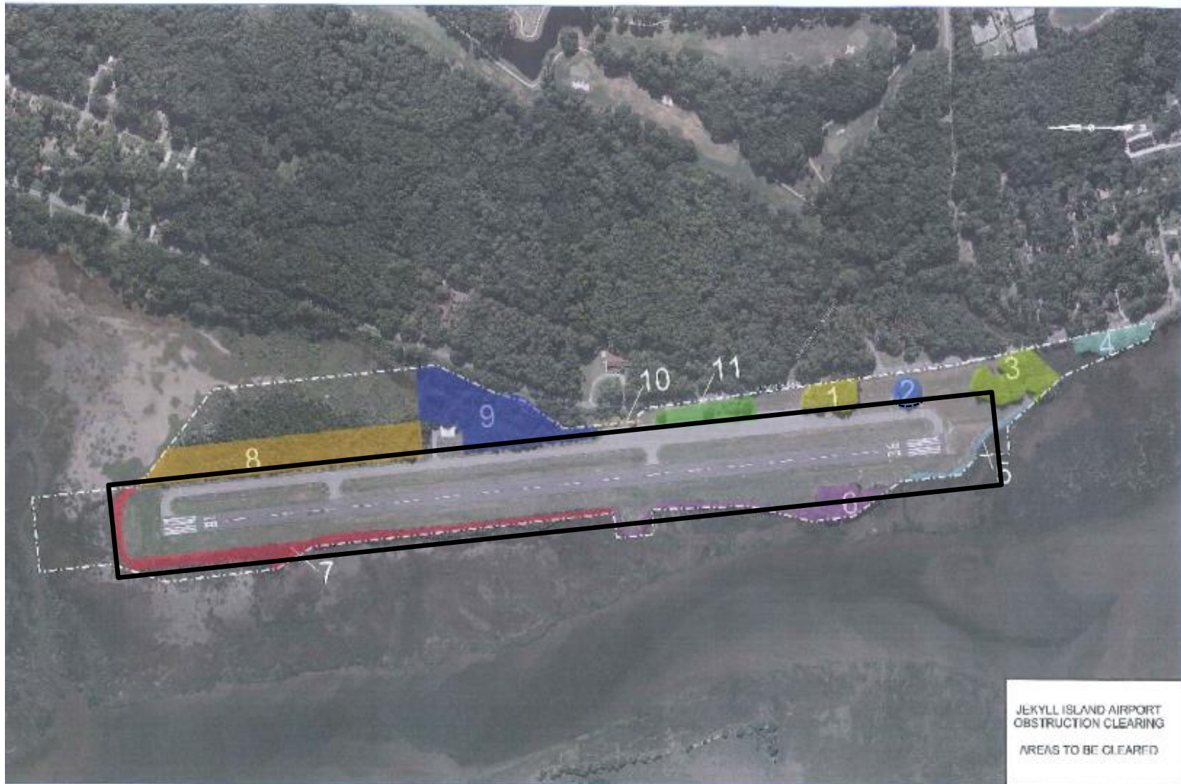
Figure 2. Proposed alternative plan: Obstruction-free zone extending 200-feet outward from either side of the runway centerline and 200-feet beyond the ends of the runway. The perimeter of the obstruction-free zone is marked by the heavy black line. The dashed black line at Zone 2 indicates a proposed exception described on page 7.
